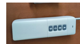
遥控开关模式 ( 双击操作, A代表升/B代表降, ) Remote control mode A indicates up, B indicates down
