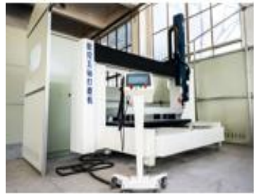
自动打磨机(*自制) Automatic grinding machine (*made by ourselves)
