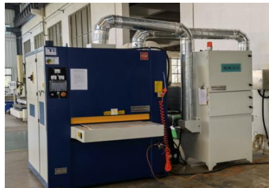
祥生金属去毛刺拉丝设备(自带除尘) Efficient metal deburring, edge rounding and finish machine
